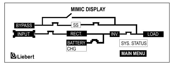
In this example, power is available from the normal and bypass sources, as well as from the battery. Notice that the switching devices are all closed except for the bypass switch at the top. The load is operating on conditioned power from the inverter. The battery is being charged by the rectifier. The static switch is operative and ready to respond to momentary demands for overload current.
